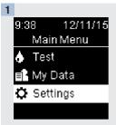
Turn the meter on by briefly pressing . From Main Menu. press to highlight Settings. Press OK
