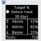
The **Target** % appears (for the **Before meal** example). The number of total tests included in the Target % appears at the bottom of the display.
