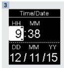
Press or to adjust each field. Press to set and move to the next field. Set am or pm if necessary.
